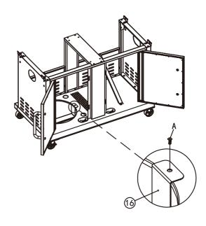
Install tank base lower (16) to the bottom shelf with 2 bolts (A).
