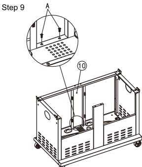
Assemble the front support (10) to bottom shelf with 2 bolts (A).
