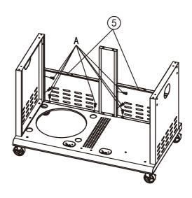
Assemble the back support (4) to bottom shelf with 2 bolts (A).
