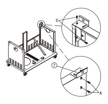
Assemble the right firebox brace (7) to the shown positions of side shelf with 2 bolts (A) and 2 bolts (C).
