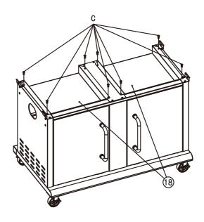
Assemble the thermal baffles (18) to the firebox brace and middle brace with 8 bolts (C) as shown.
