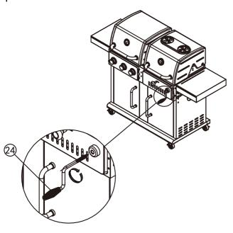
Screw the lifting handle (24) to the control panel twist clockwise.
